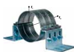
Point fixe 3 colliers Charge admissible maxi. axiale F_a = 16500 N radiale F_r = 13980 N
